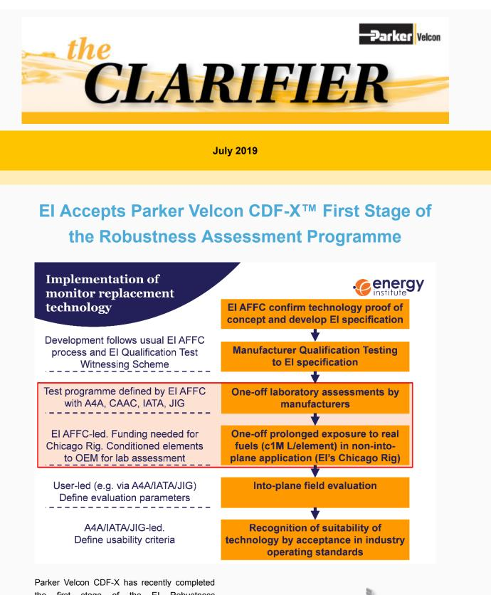
the first stage of the EI Robustness Assessment Programme. On July 8th, the EI Aviation Fuel Filtration Committee concluded that the results support model CDFX-2xxA water barrier elements being suitable for Stage 2 robustness testing.
